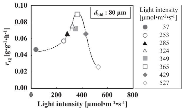
**Fig. 3** Association between light intensity and  $r_{\text{sg}}$  in the semi-batch photobioreactor
