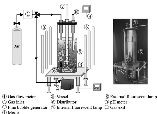
Fig. 1 Outline of the semi-batch photobioreactor equipped with a self-supporting bubble generator
