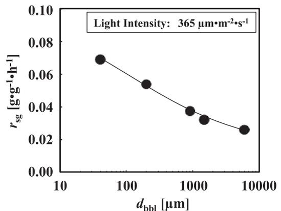
**Fig. 4** Association between  $d_{\text{bbi}}$  and  $r_{\text{sg}}$  in the semi-batch photobioreactor
