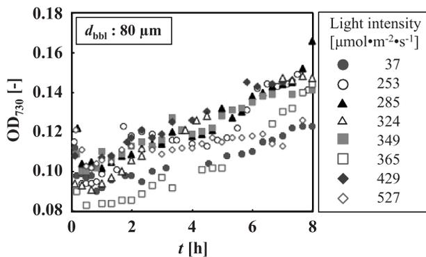
**Fig. 2** Light intensity-dependant changes of  $\text{OD}_{730}$  in continuous bubbling ( $d_{\text{bbi}}: 80 \mu\text{m}$ )
